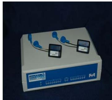
Fig.2: *ZeroWire* EMG: completely wireless system for surface EMG.
