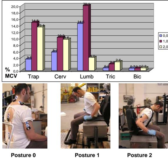
Fig.3: mean value of muscles activation (at % MCV) in postures 0, 1 and 2 were Trap= upper trapezius, Cerv= cervical erector spinae, Lumb= lumbar erector spinae, Tric= triceps, Bic= biceps.
